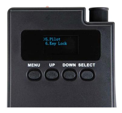
**5. Pilot** Activates or deactivates Pilot Tone for use with compatible transmitters.
